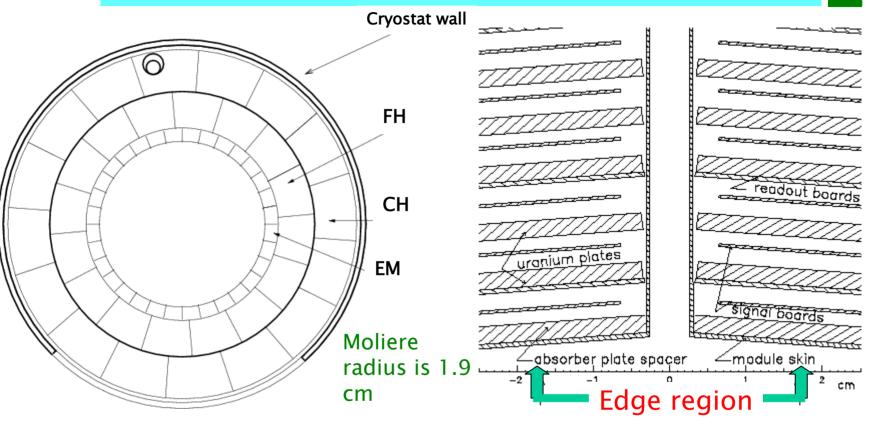
most DØ exclude electrons 1.8 cm from module edges (10% of width)
